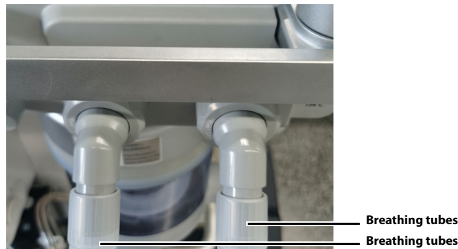
Figure 11-35 Install the breathing tubes
