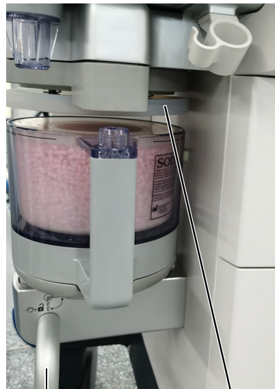
Unlocking position. The bypass is turned on.
