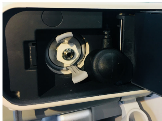
Figure 11-32 Insert the O 2 sensor support to the breathing system
