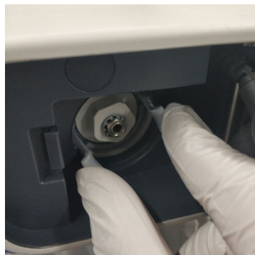
Figure 11-6 Remove the O 2 sensor support from the breathing system
