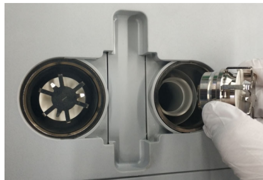
Figure 11-16 Remove the inspiration and expiration valves
