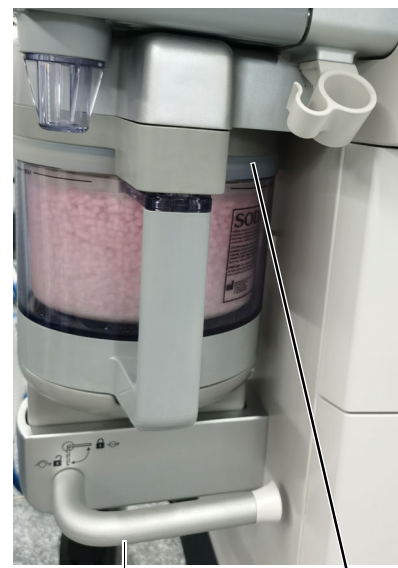
Locking position. The bypass is turned off.
