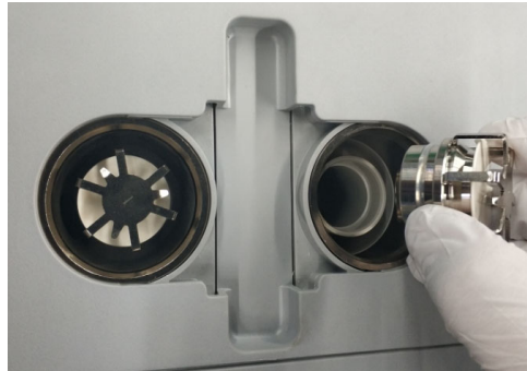
Figure 11-21 Insert the inspiration and expiration valves
