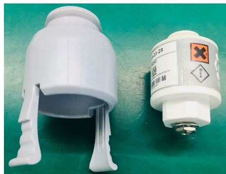
Figure 11-7 Remove the O 2 sensor from the support
