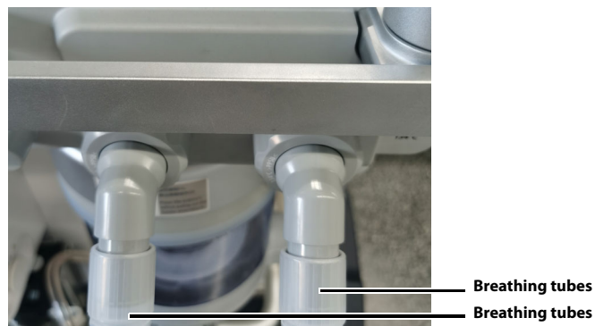
Figure 11-2 Remove the breathing tubes
