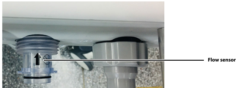
Figure 11-25 Install the flow sensor
